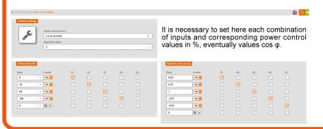
If you want to use power control module for other Solar Monitor units, which are in the same net as the unit, which the module SM2-PC is directly connected to, choose the possiblity "Remote" in "Power control source". It is not necessary to connect the module SM2-PC to these units. Controlling is under way of the local module configuration.
