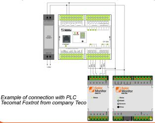
This picture shows the example of the connection for active power control in steps 0 - 30 - 60 - 100%.
