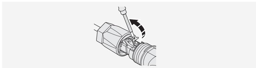
4) Insert the stripped DC cable to the battery connector deep enough and toggle the clamping bracket to make sure it tightly locked with the stripped cable.
