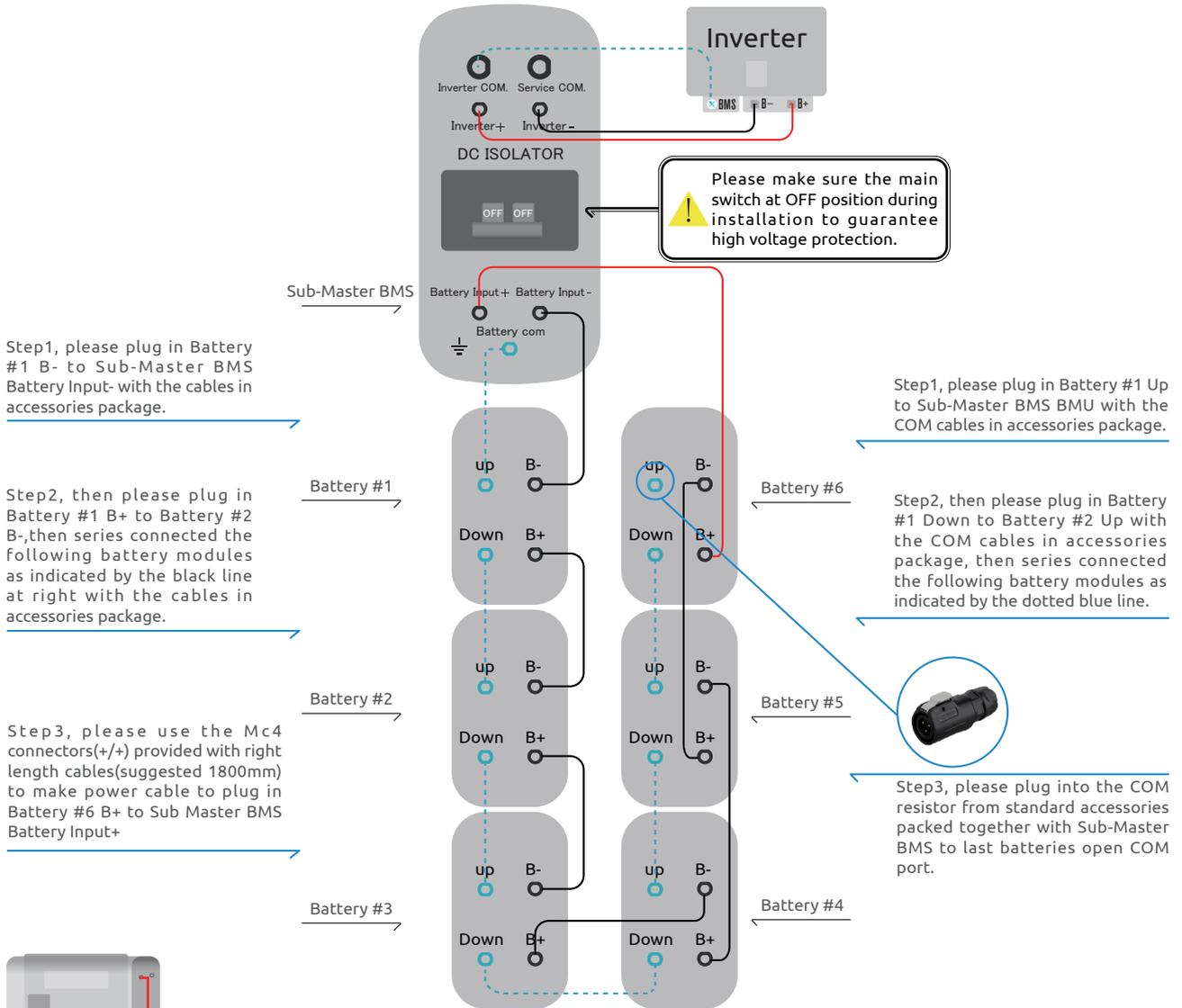
Step1, please plug in Battery #1 B- to Sub-Master BMS Battery Input- with the cables in accessories package.
