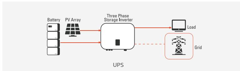
\* During UPS mode, if battery long time no discharge, the inverter will discharge and charge battery periodically(every 1 week) with small current roughly 1A to reset battery SOC.
