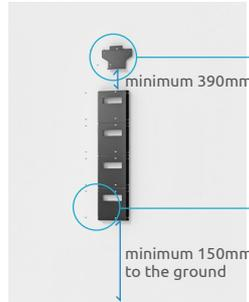
Please use 7pcs Inverter back sheet expansion screws to fix the Inverter's back sheet to wall.
