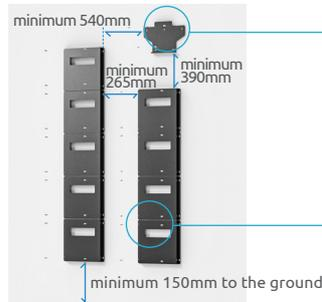
Please use 7pcs Inverter back sheet expansion screws to fix the Inverter's back sheet to wall.
